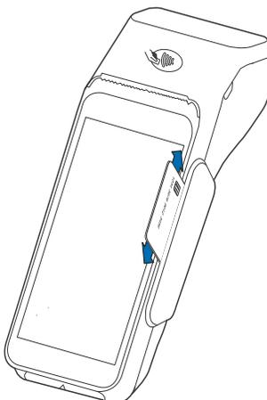
**Figure 12 Using Magnetic Stripe Card**
