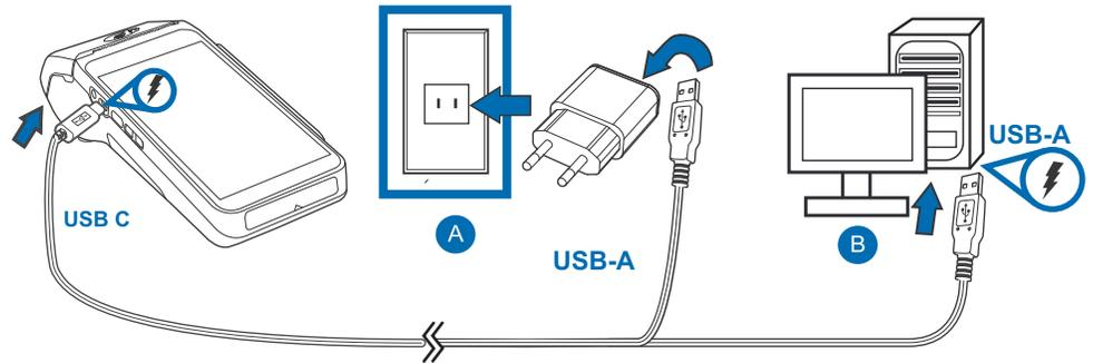
**Figure 9 T650p Power Supply Connection**
