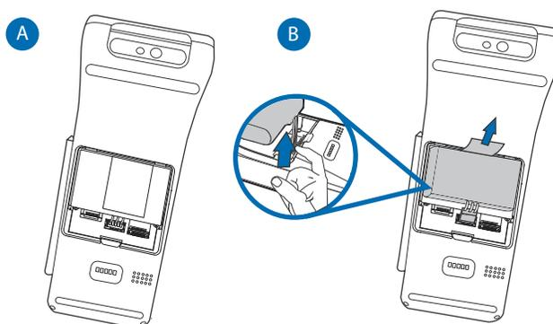
**Figure 5** Removing Battery
